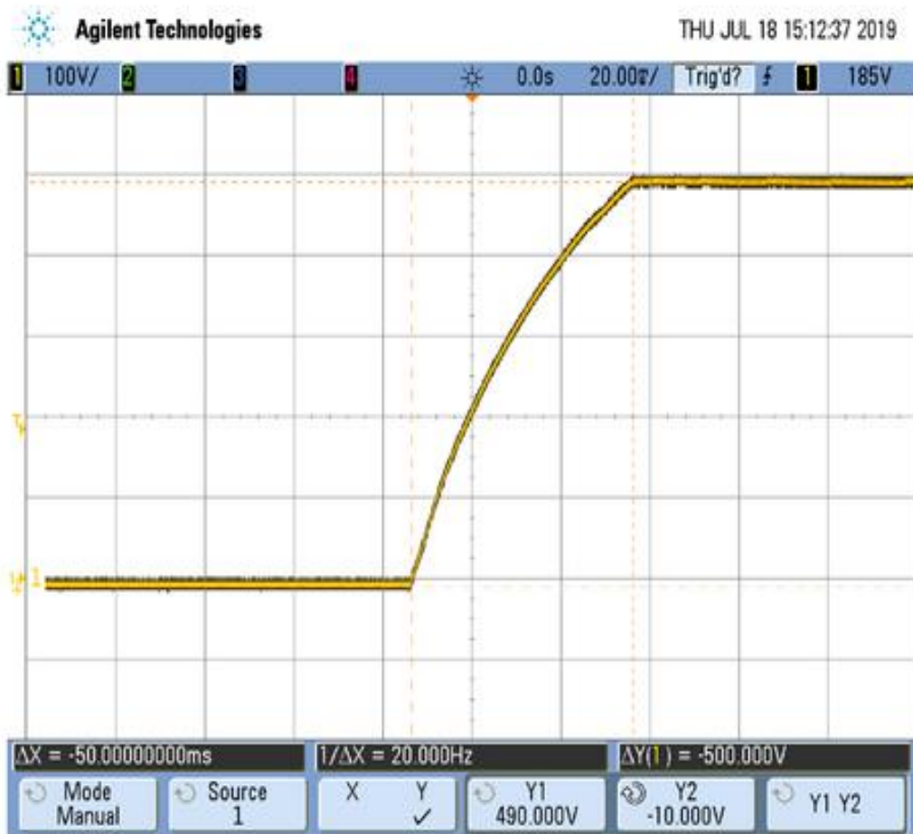
Fig. 7 – Capacitor voltage oscillogram measured during quasi constant power charging
