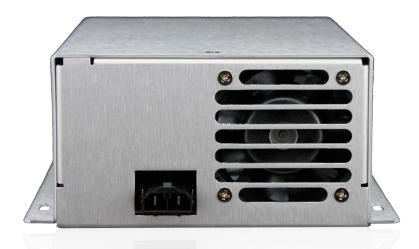
The HPP-750 laser diode pulser is a new concept in pulsed diode driver development. Designed to be used with the LDD series drivers as the power source, the HPP-750 pulser can deliver up to 350 amps of output current with full protection of the laser diode. Pulse widths of ≥50µs to CW can be acheived with rise/fall times of <10µs. and repetition rates to 5kHz.
